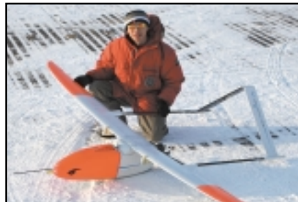
Most UAV systems have been designed, built, and flown in the desert. Few have been designed for the rigours of Canada's northern climate. This Small UAV, the Aerosonde, has successfully flown 1000+ mission hours in the Arctic – in severe icing conditions and temperatures dropping to -35°C.
