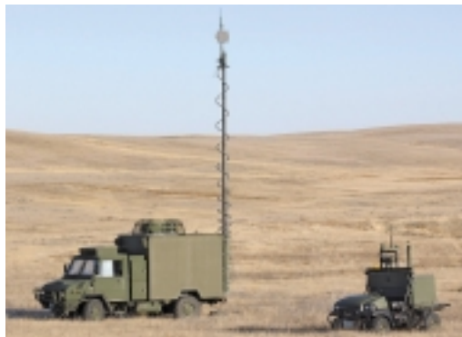
MATS Unmanned Ground Vehicle & LSVW Command Post with data link mast deployed.
