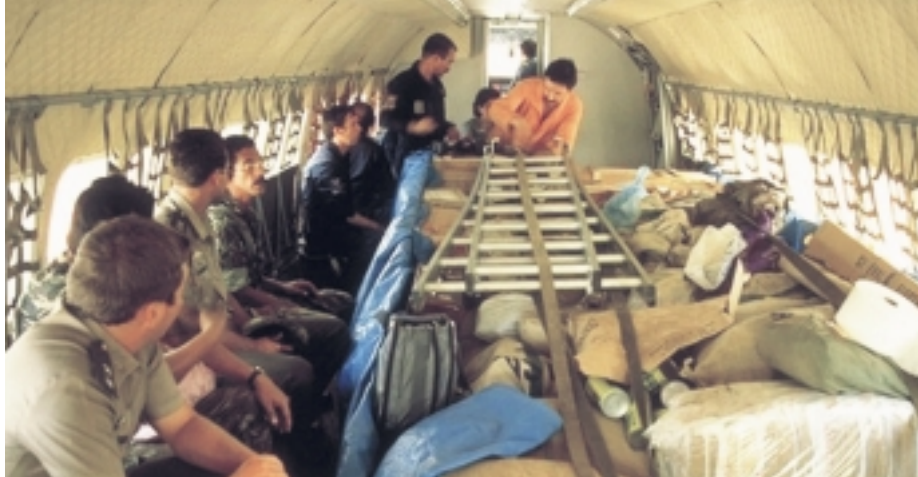
During the recent demo tour, pilots, SAR Techs, Spotters and CASARA volunteers were impressed with the features of the C-295. Deceptively streamlined on the outside, many were surprised at the fully stand-up cabin, the unique capability to carry three standard pallets, and the extra space for consoles, Sar Techs, Spotters, stretchers, or two additional pallets.
